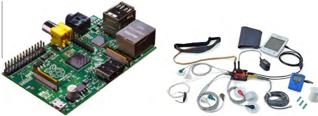
Fig. 16. Raspberry Pi e-Health kit showing a range of connectable sensors and devices.
