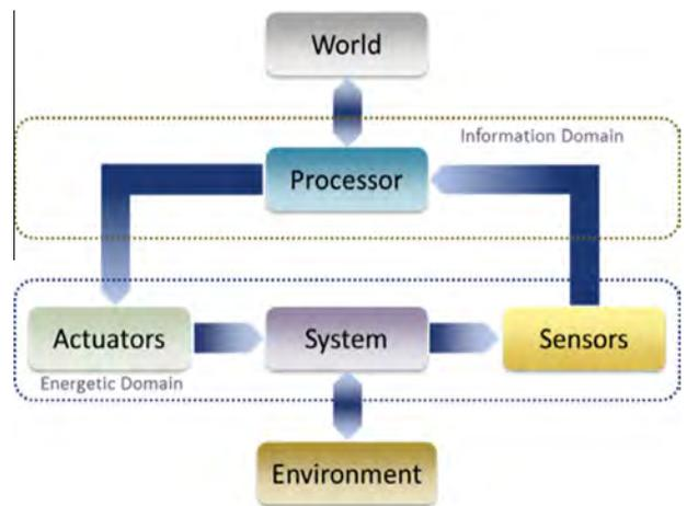
Fig. 5. A conceptual model of a conventional mechatronic system.
